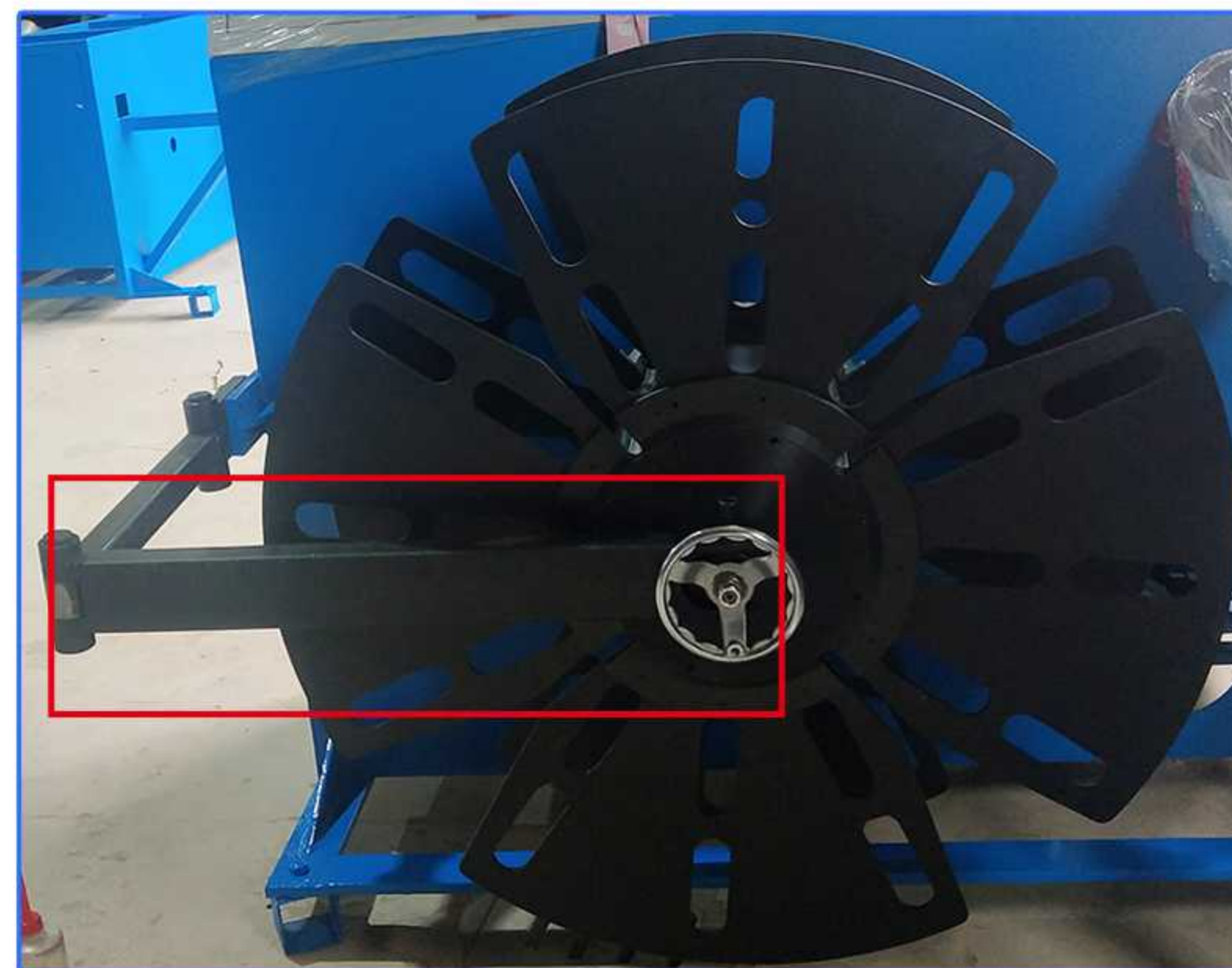
A support to stabilize the coil
