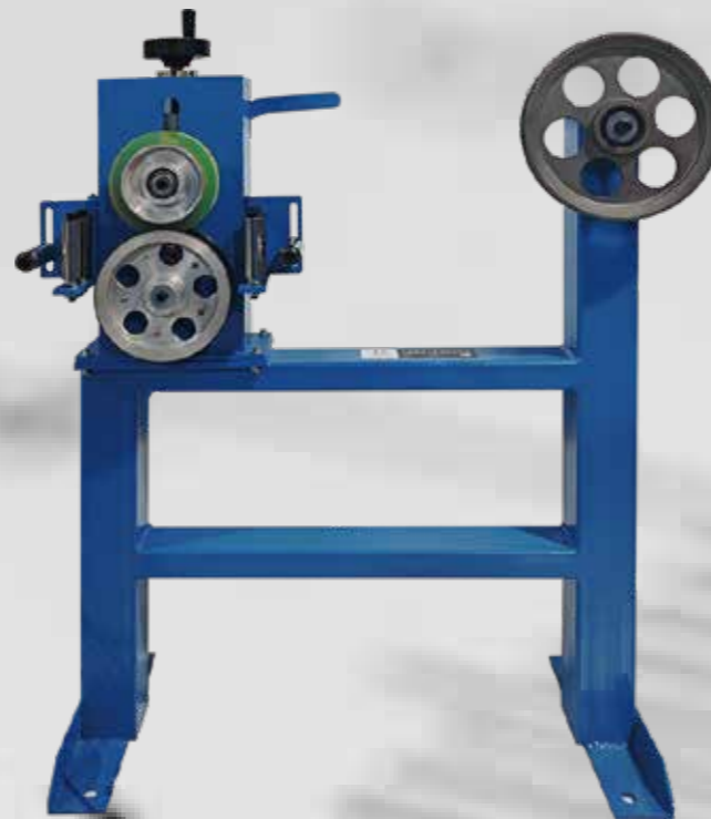
QP-30成圈机专用计米器 QP-30 Length Meter Counter for Take-up Machine
